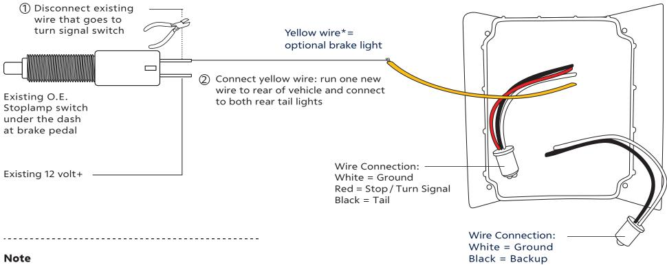
This will disable the "sequence once" brake attention feature. Do not use this instruction if the vehicle is used for towing and trailer lights.
